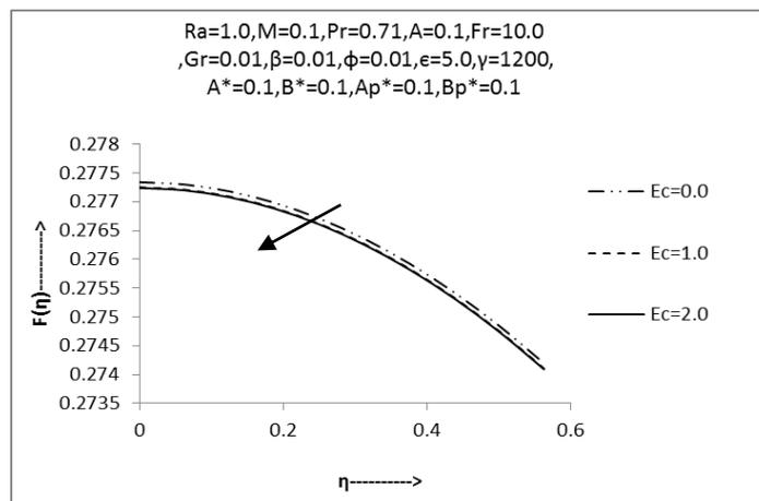
**Fig.5: Non-dimensional velocity profile of particle phase w.r.t. 'Ec'**
