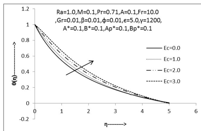
**Fig.6: Non-dimensional temperature profile of fluid phase w.r.t. 'Ec'**
