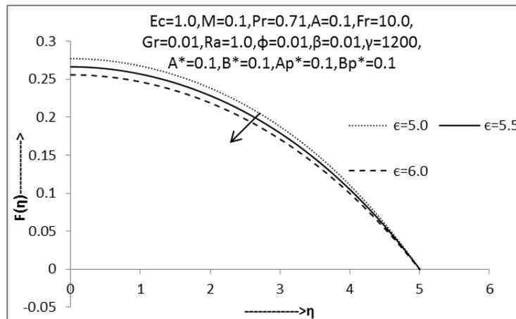
Fig.29: Non-dimensional velocity profile of particle phase w.r.t.  $\epsilon$
