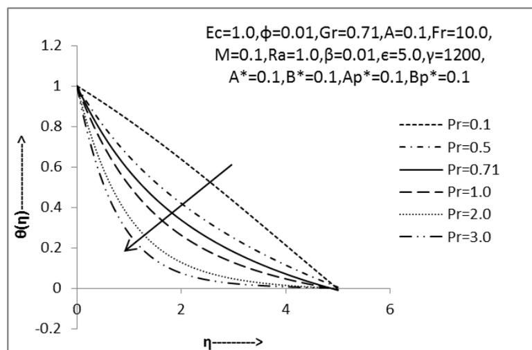
**Fig.21: Non-dimensional temperature profile of fluid phase w.r.t. 'Pr'**
