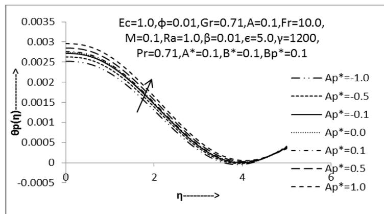
Fig.27: Non-dimensional temperature profile of particle phase w.r.t. ' $Ap^*$ '
