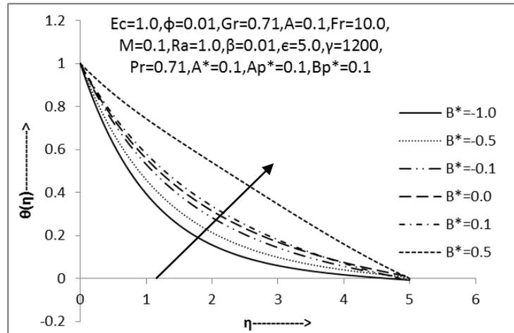
Fig.25: Non-dimensional temperature profile of fluid phase w.r.t. ' $B^*$ '
