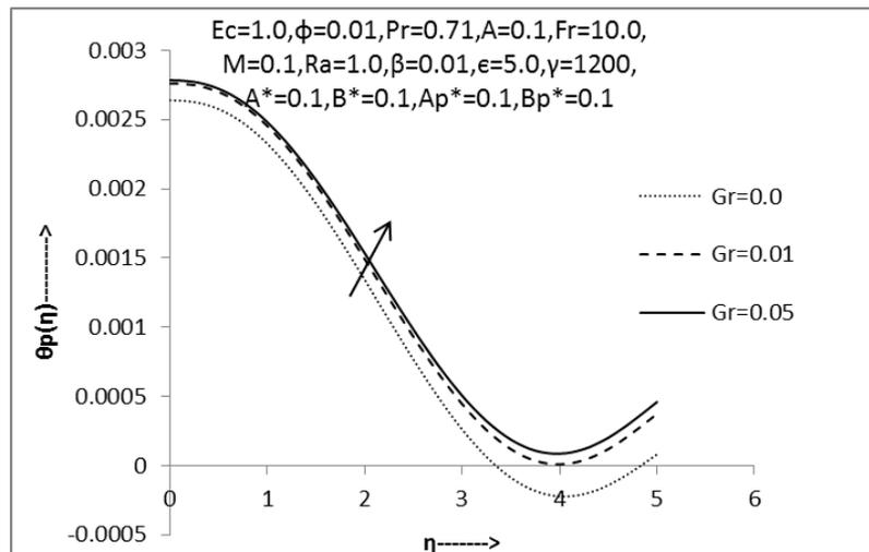
**Fig.19: Non-dimensional temperature profile of particle phase w.r.t. 'Gr'**
