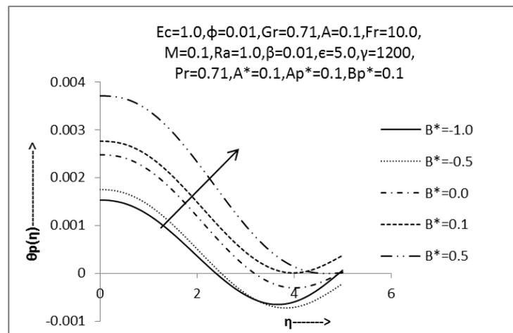
Fig.26: Non-dimensional temperature profile of particle phase w.r.t. ' $B^*$ '
