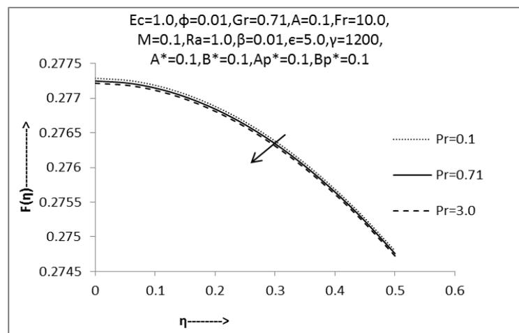
**Fig.20: Non-dimensional velocity profile of particle phase w.r.t. 'Pr'**
