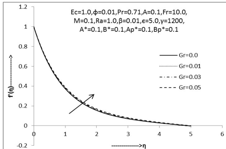
Fig.16: Non-dimensional velocity profile of fluid phase w.r.t. 'Gr'
