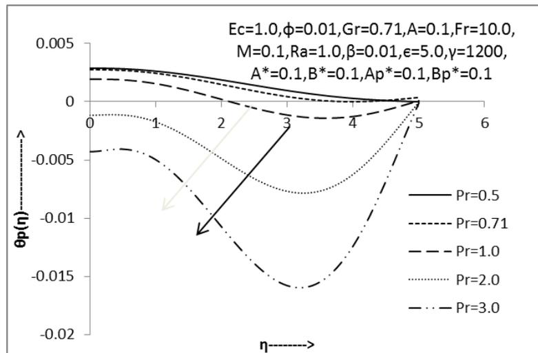
Fig.22: Non-dimensional temperature profile of particle phase w.r.t. 'Pr'
