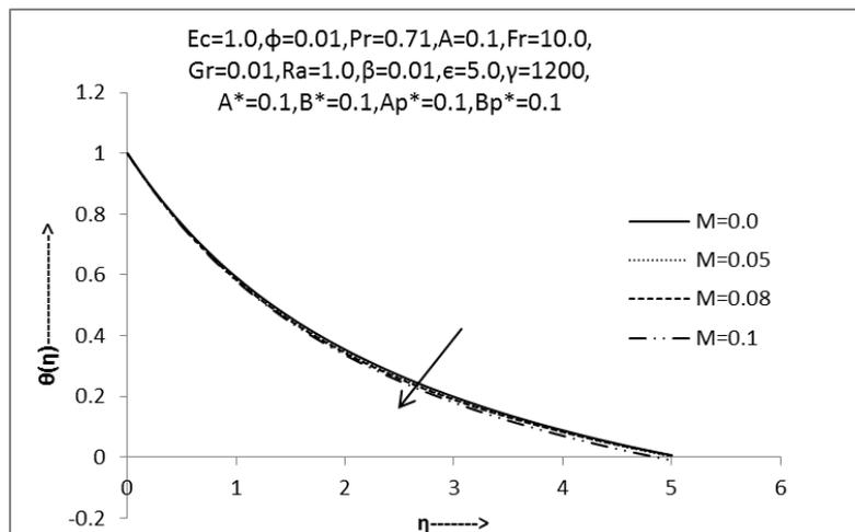
Fig.15: Non-dimensional temperature profile of fluid phase w.r.t. 'M'
