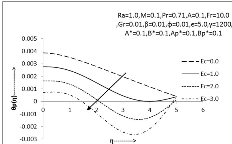
Fig.7: Non-dimensional temperature profile of particle phase w.r.t. 'Ec'
