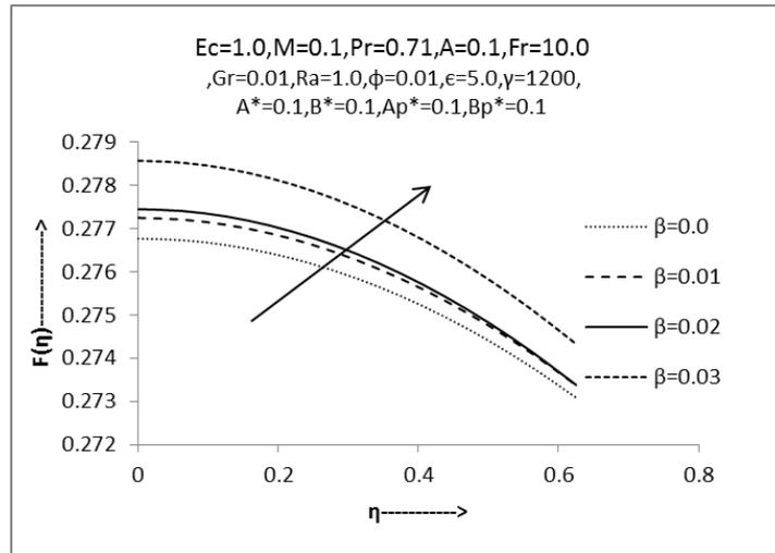
Fig.10: Non-dimensional velocity profile of particle phase w.r.t. 'β'
