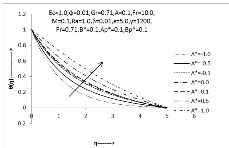
Fig.23: Non-dimensional temperature profile of fluid phase w.r.t. 'A\*'
