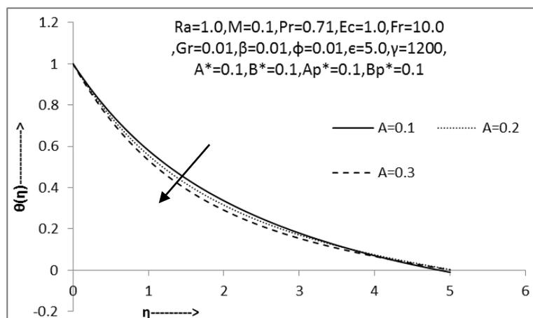
Fig.3: Non-dimensional temperature profile of fluid phase w.r.t. 'A'
