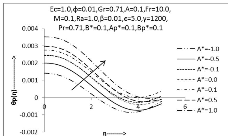
Fig.24: Non-dimensional temperature profile of particle phase w.r.t. 'A\*'
