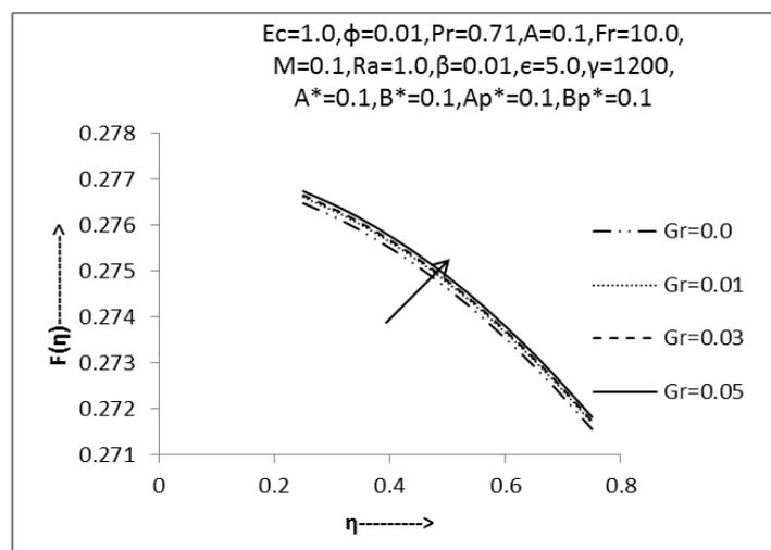
Fig.17: Non-dimensional velocity profile of fluid phase w.r.t. 'Gr'
