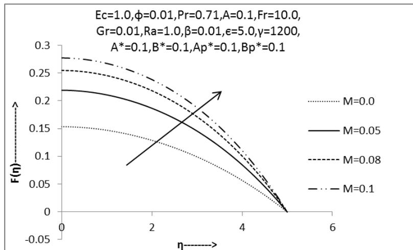
Fig.14: Non-dimensional velocity profile of particle phase w.r.t. 'M'
