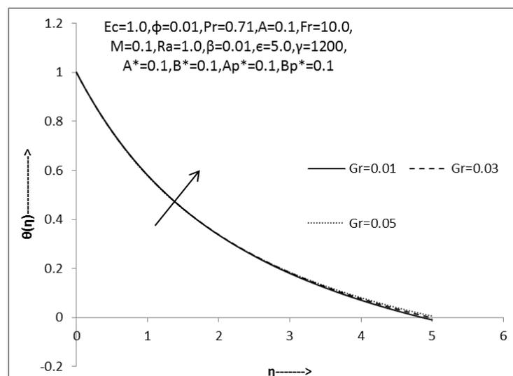
Fig.18: Non-dimensional temperature profile of fluid phase w.r.t. 'Gr'
