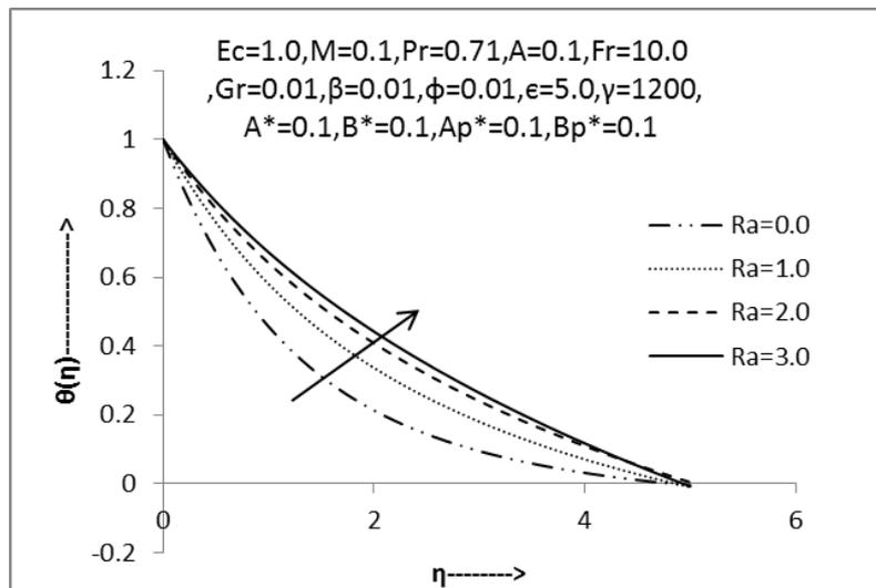
Fig.8: Non-dimensional temperature profile of fluid phase w.r.t. 'Ra'
