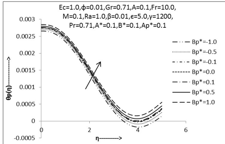
Fig.28: Non-dimensional temperature profile of particle phase w.r.t. 'Bp\*'
