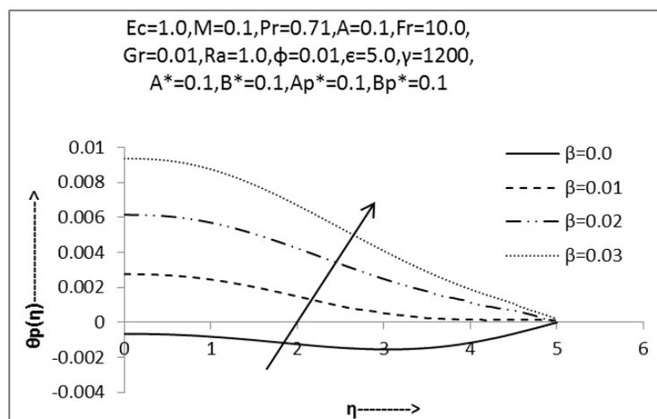
Fig.12: Non-dimensional temperature profile of particle phase w.r.t. 'β'
