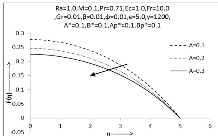
Fig.2: Non-dimensional velocity profile of particle phase w.r.t. 'A'
